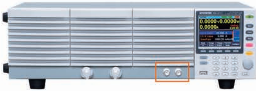
BNC connectors on the front panel
